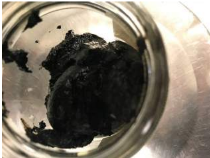
Photo 10: Dewatered solids from geotube
