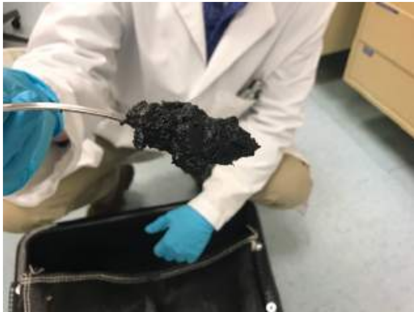
Photo 9: Dewatered solids from geotube
