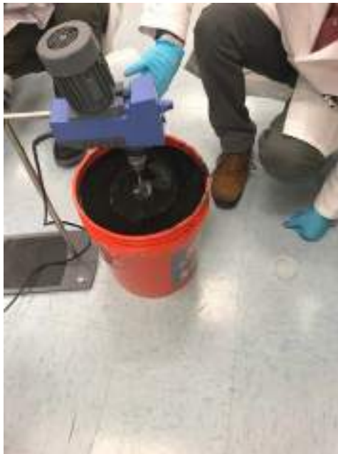
Photo 1: Mixing of sample with amendments for geotube
