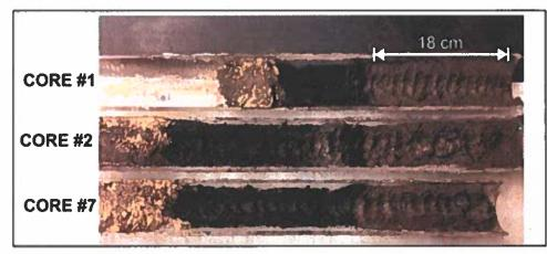
This image shows several core samples taken from Boat Harbour, the black contaminated sludge is clearly visible; the brownish gray is the clean Preindustrial marine sediment and, the bentonite is a clay product put in the core during sampling as a plug - Note: The figure shows from left to right bentonite plug, black contaminated sludge, brownish gray pre-industrial marine sediment
