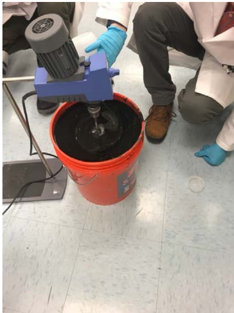
Photo 1: Mixing of sample with amendments for geotube
