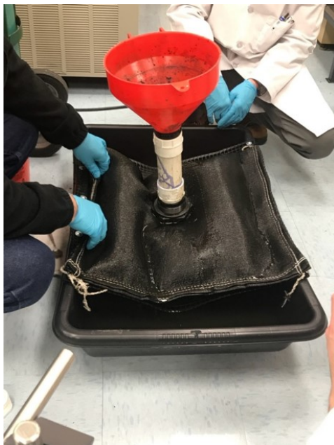
Photo 1: Mixing of sample with amendments for geotube
