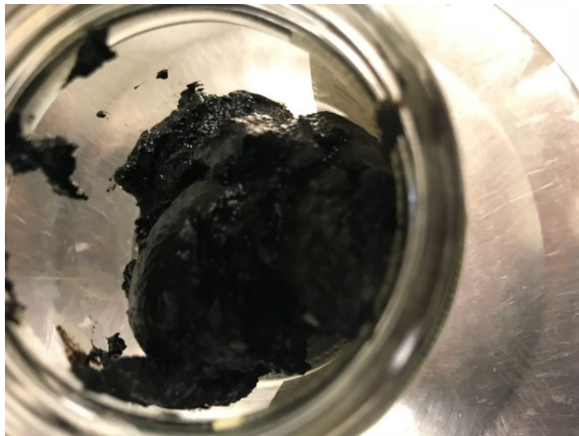
Photo 10: Dewatered solids from geotube
