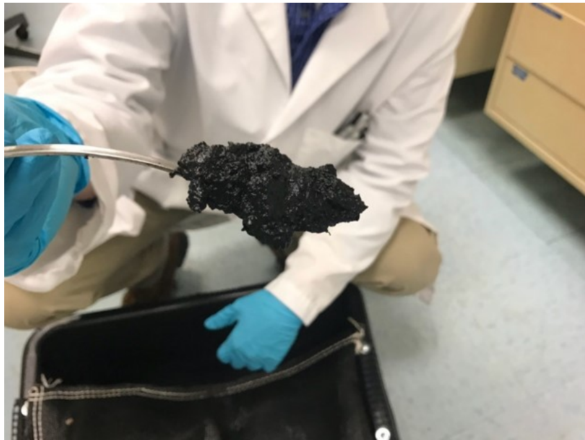
Photo 9: Dewatered solids from geotube
